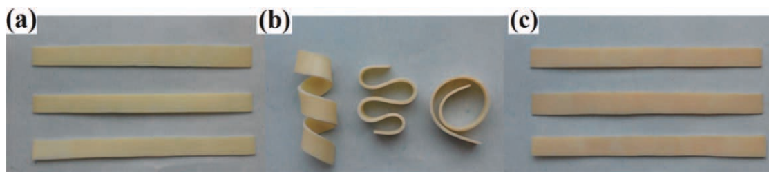
Figure 9. Visual demonstration of shape memory properties for 30%SEP-80 (a: original/permanent shapes, b: fixed temporary shapes, c: recovered shapes). [Color figure can be viewed in the online issue, which is available at wileyonlinelibrary.com .]
